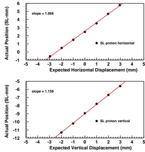
Figure 4: The horizontal and vertical proton beam displacements as measured by Synclite versus the calculated expected displacements.
