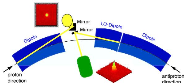
Figure 1: Synclite schematic showing radiation point locations for protons and antiprotons.
