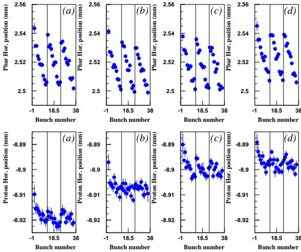
Figure 5: Horizontal positions of each of the 36 bunches for antiprotons (top) and protons (bottom), where (a, b, c, d) give the averaged positions for 0–20, 20–40, 40–60 and 60–80 minutes after the start of collisions for a collider store.
