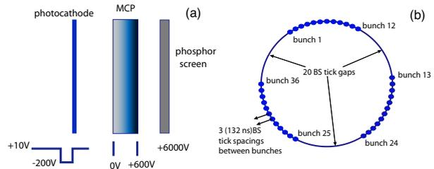
Figure 2: (a) Schematic of image intensifier showing the typical high voltages used; (b) Schematic of beam in the Tevatron illustrating the time structure for the 36 proton bunches. The 36 antiproton bunches have a similar time structure.
