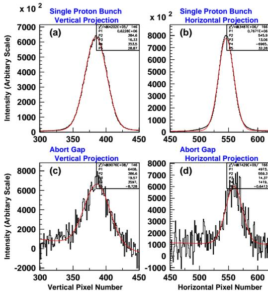
Figure 6: (a,b) Vertical and horizontal projections of the background subtracted image for a single  $1.8 \times 10^{11}$  proton bunch at normal MCP high voltage; (c,d) Vertical and horizontal projections of the background subtracted image for a 670 ns time interval in the beam abort gap. The projections are fit with a Gaussian signal and a linear background function.
