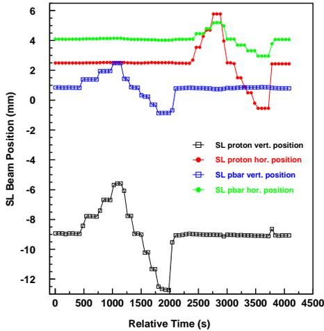
Figure 3: The horizontal and vertical locations of the proton and antiproton beams as measured by Synclite versus time, for the time period when the beams were bumped vertically then horizontally.
