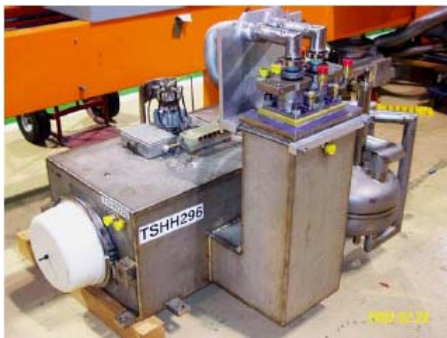
Figure 4-10: modified H-spool with HTS lead package on the floor at MTF.
