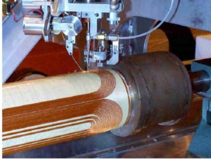
Figure 4-6: Photograph of BNL Direct Wind corrector fabrication in process.
