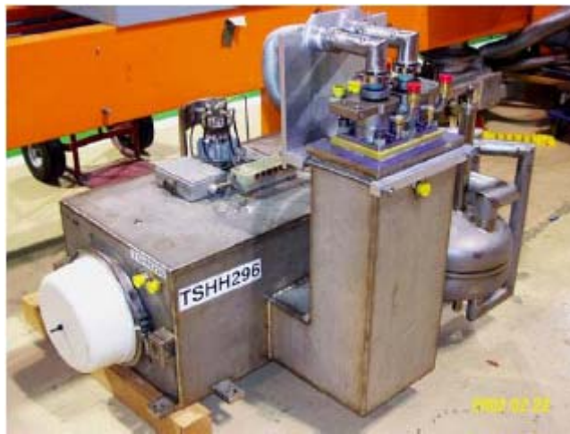
Figure 4-8: modified H-spool with HTS lead package on the floor at MTF.
