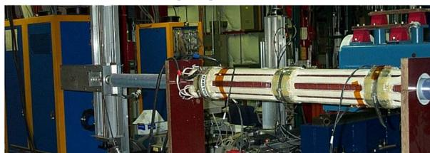
The air-core quadrupole was modified to fit on a 4" beam pipe. Above it is being measured in the Magnet Test Facility (MTF) using a rotating coil.
