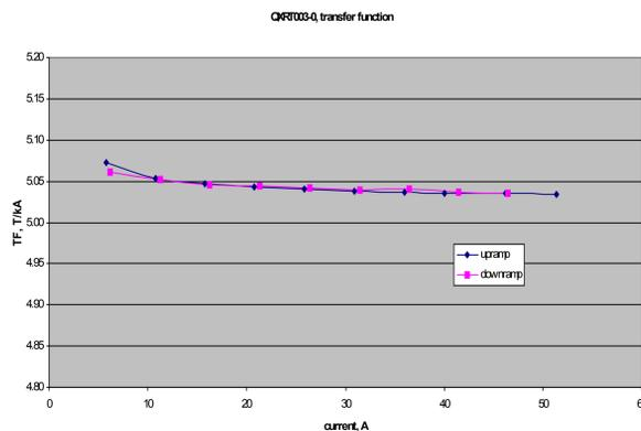
Measured transfer function (integrated gradient per unit current).
