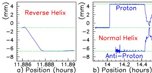
Figure 4. Comparison of antiproton position with that of protons on the reversed helix, for BPM VA35. The time axis is time of day, in hours
