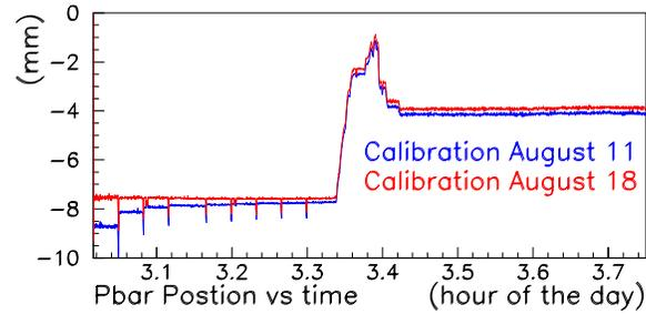
Figure 4. Antiproton data from August 18, processed using two different calibrations for the cancellation coefficients. The time axis is time of day, in hours
