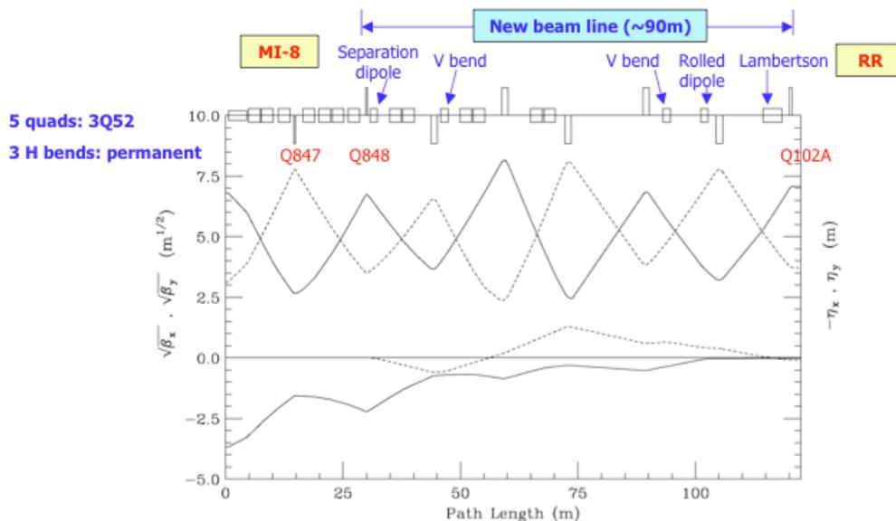
Figure 2 – Example solution for MI-8 beam line re-matched for Recycler injection.
