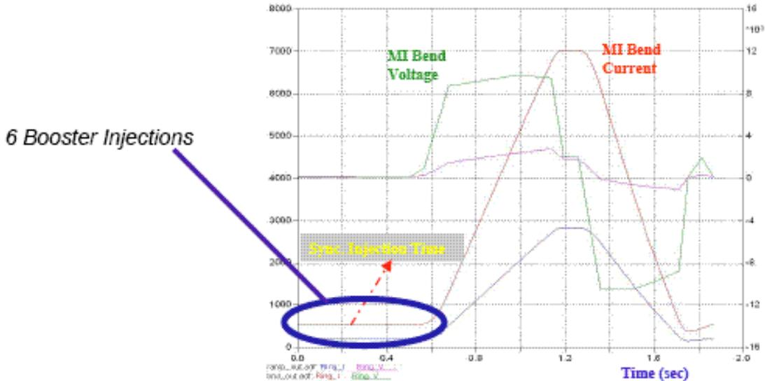
Figure 1 – Present Main Injector cycle, showing dwell time for 6 Booster injections.
