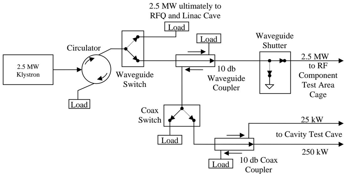
Figure 1. RF Power Distribution System
