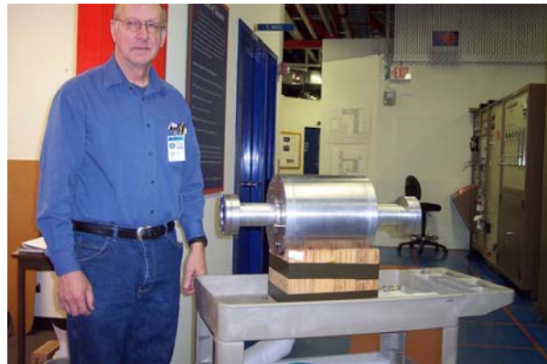
Fig. 7: Model RF showing the moveable sleeves that allow the separation of the irises to be changed.
