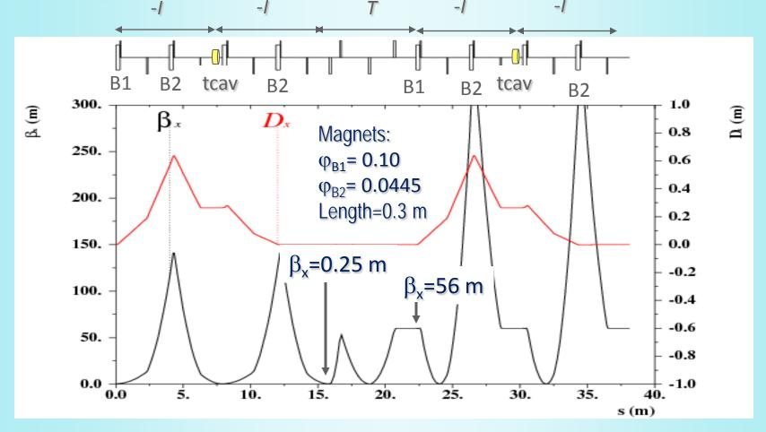
Lattice functions for a bunch compressor with a telescopic factor m=15. Note, matching of the vertical beta-function was not pursued.
