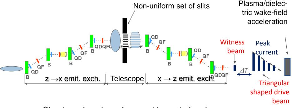
Shaping e-bunch peak current to control and prepare a coherent wake-field excitation
