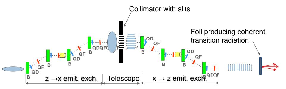
Using demagnification of the beam size before slits and magnification after the slits can help to obtain a real tight spacing of microbunches
