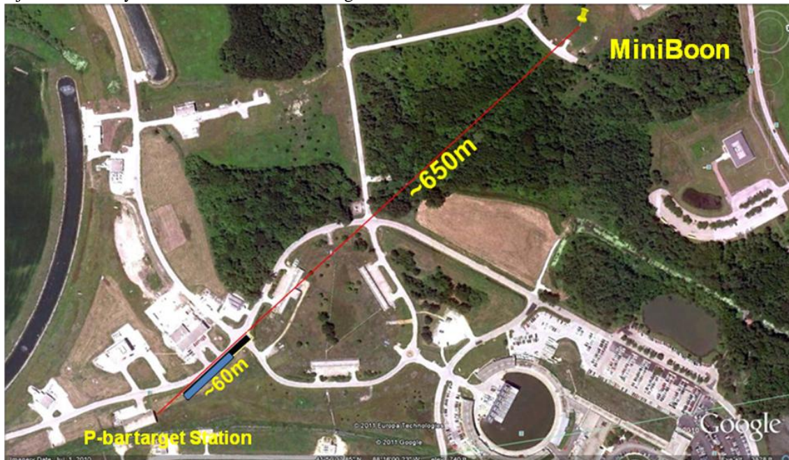
Figure 1: Fermilab, Antiproton Complex, with racetrack storage/decay ring depicted as blue box. The red line indicates direction of neutrino beam that hits MiniBoon detector.
