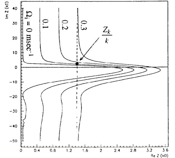
Fig.1. Instability curves showing graphical solution of growth rate.
