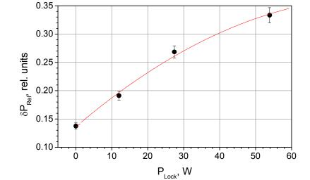
Measured allowable range of the power control of the magnetron vs. the pre-exciting power.
