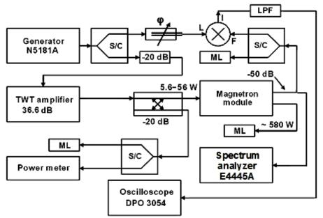
Experimental setup to measure the magnetron current, voltage, spectrum, output power, power of the pre-exciting (frequency-locking) signal and phase noise. The measurements in pulsed mode were performed at 2.7 MHz shift of the frequency locking the magnetron.
