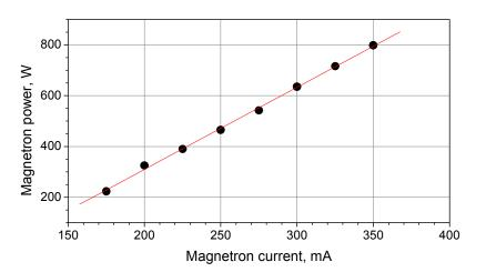
The measurements in CW mode were performed at the frequency locking the magnetron approximately equal to average frequency at free run at magnetron power of ~800 W.
