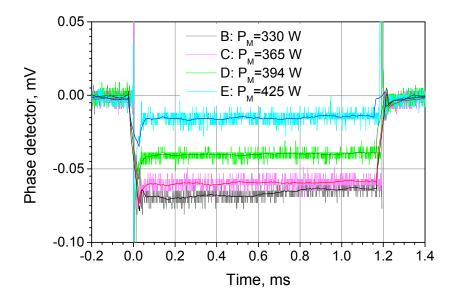
Measured by the phase detector stochastic noise at various magnetron power. Calibration is 2.4 mV/degree.
