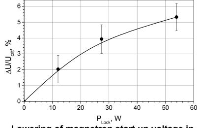
Lowering of magnetron start up voltage in percents vs. the power of signal,  $P_{Lock}$ , pre-exciting the magnetron.
