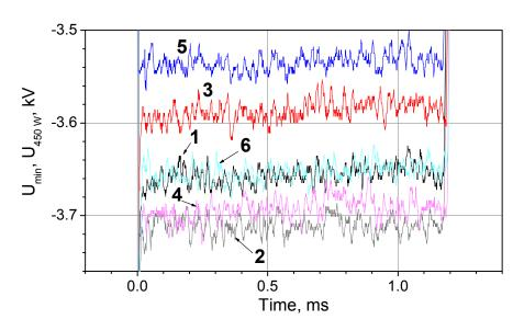
Pulsed cathode voltage at minimum generated power, traces 1, 3, 5, and at power of 450 ±8 W, traces 2, 4, 6 at the following powers of the frequency-locking signal,  $P_{Lock}$ : 12 W, traces 1 and 2, 27.4 W, traces 3 and 4, 53.9 W, traces 5 and 6, respectively. Minimum amplitude of the free running magnetron is 3,737±9 V
