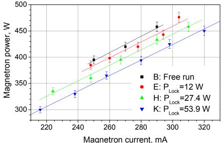
Dots with error bars: dependence of the magnetron pulsed power on the magnetron current vs. power of pre-exciting signal. Solid lines: linear fits of the measured data.
