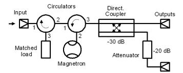
The magnetron assembly to study the power control.
