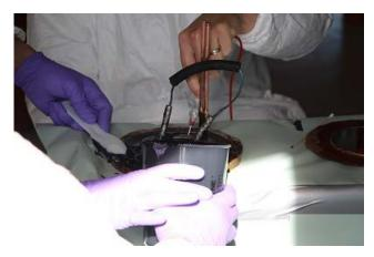
11.4 Insert the cone plug by hand and tap into place. Clamp the plug in place just above the foil fingers on each \*cone. Wipe off any excess epoxy from the plug and clamp.
