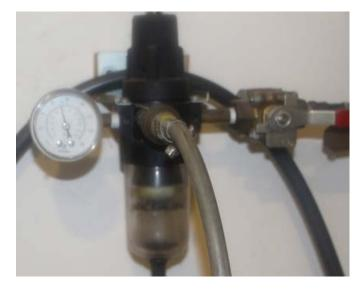
NOTE: Set compressor to proper setting for spray gun 50 -  $70 \, PSI$
