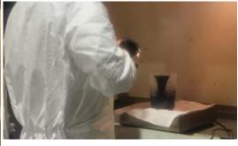
8.5 Blend by hand, using a kneading motion, for 2-3 minutes scraping the sides and bottom of the container frequently.
