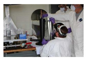
11.2 Carefully slide the Foil Sector Assembly onto the Cooling Cone without allowing the Foil Sector Assembly to scrape the Epoxy mixture from the Cooling Cone. The bottom edge of the Foil Sector Assembly and the Cooling cone should be flush. If tight, the Cooling Cone may extend out from the Foil Sector Assembly up to 3/16"
