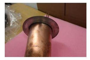
7.3.2 Inspect the copper foils for damage large dents, creases, pin holes, etc. Inspect the interior welds for large protrusions or material buildup. If defects are not excessive, the joints may be carefully dressed with a file. Tape copper foil as shown in illustration. All three interior seams, both sides of the flange, and the fingers/grooves must be taped as shown. Ensure tape has been pressed closely into welds, minimize trapped air under the taped seams.
