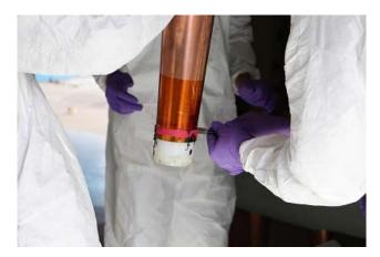
11.5 Bring the assembly under vacuum to eliminate air pockets in assembly. Back fill with additional Epoxy and repeat as necessary.
