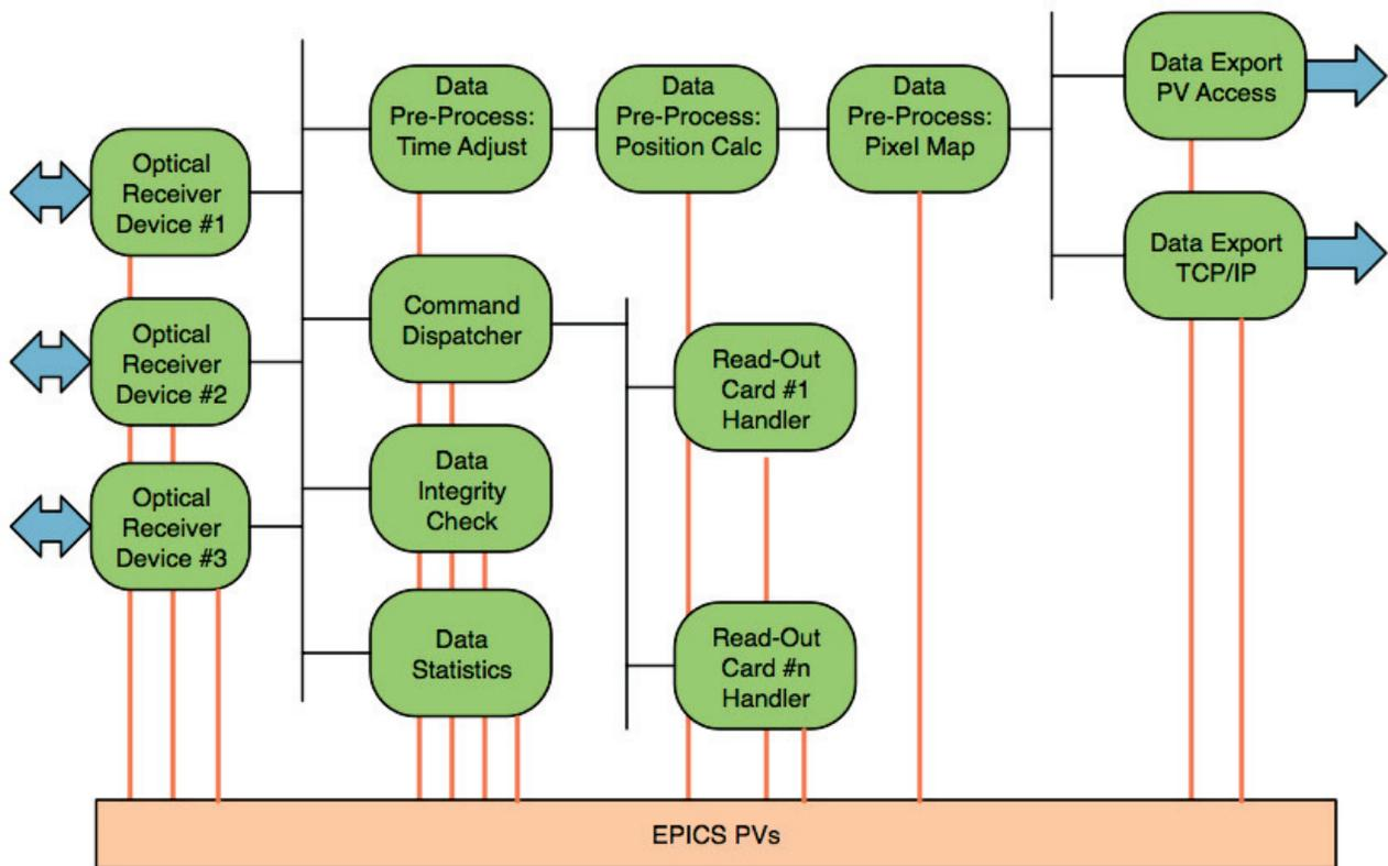
Figure 2: The nED modular design allows arbitrary plug-in connections, from any plug-in to any other plug-in, for numerous configuration possibilities
