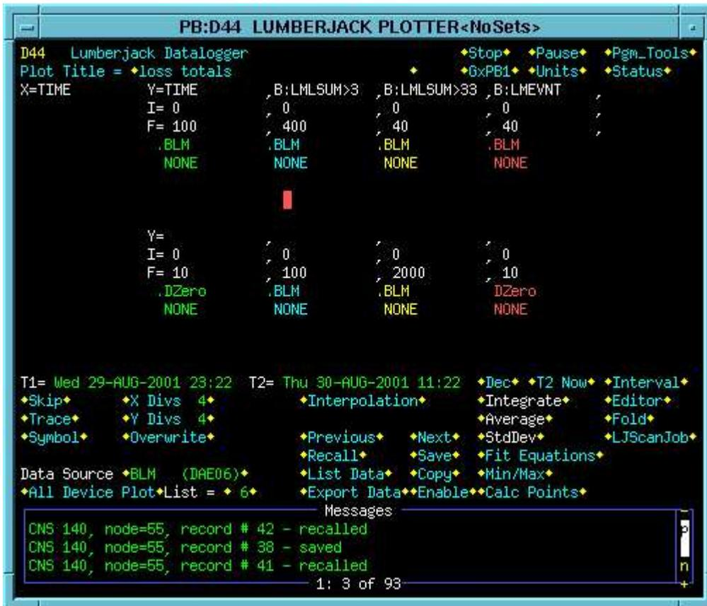
The yellow and cyan traces indicate the change in charge accumulators between two collections at millisecond markers 33 and 3 respectively. The red trace indicates reset event 20. (0x14) as well as reset events 0x17 and 0x1B.
