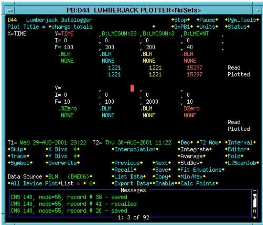
The yellow and cyan traces indicate the change in charge accumulators between two collections at millisecond markers 3 and 33 respectively. The red trace indicates reset event 20. (0x14) as well as reset events 0x17 and 0x1B.
