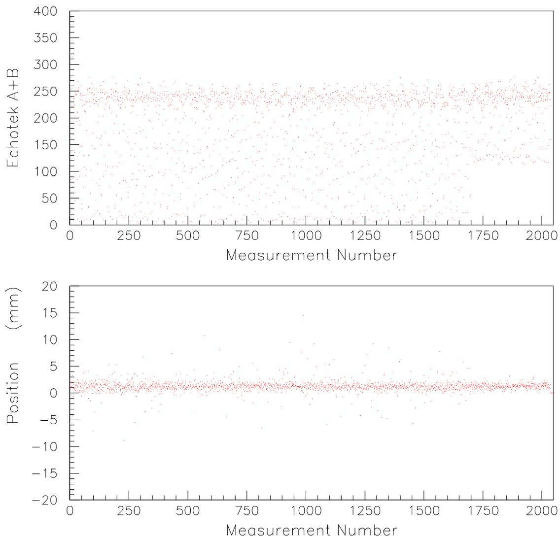
Figure 4: These plots show 2048 consecutive points from a hand triggered turn by turn measurement. The measurement was triggered by hand, without any reference to any timing signals. I believe, but can't really prove, that there was indeed beam in the machine for this measurement. There is clearly a big problem with the sum signal and there are significant outliers in the position signal. See the text for details.
