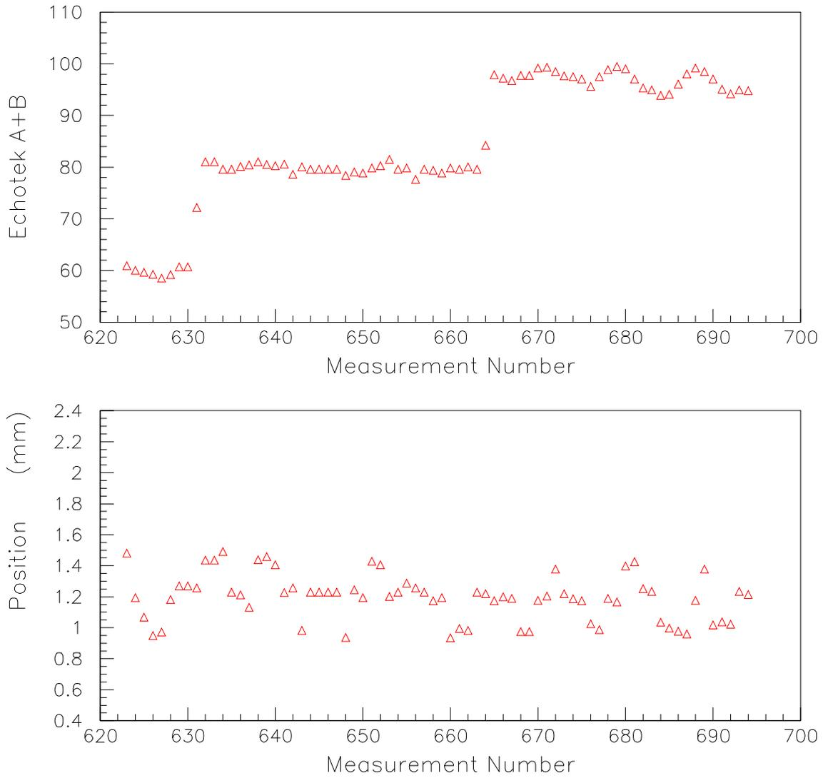
Figure 3: These two plots show details of the upper two plots in the previous figure. The period selected for detail is that used to measure the resolution (between the vertical blue lines). The position appears to be quantized and I interpret this as evidence that we are seeing the granularity of the Echotek.
