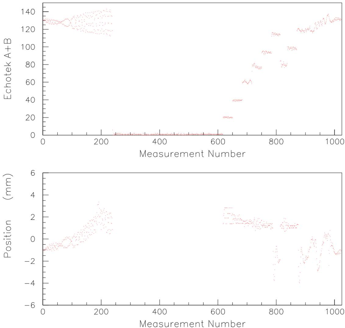
Figure 1: These plots show 1024 consecutive closed orbit measurements taken with the MI BPM test equipment in MI40. The points were recorded at 500 Hz, which means that the horizontal axis covers about 2 seconds. The start time was not synchronized with any timing signal. The upper plot shows the sum signal ( $|A| + |B|$ ) plotted against measurement number. The lower plot shows the position, in mm, plotted against measurement number.
