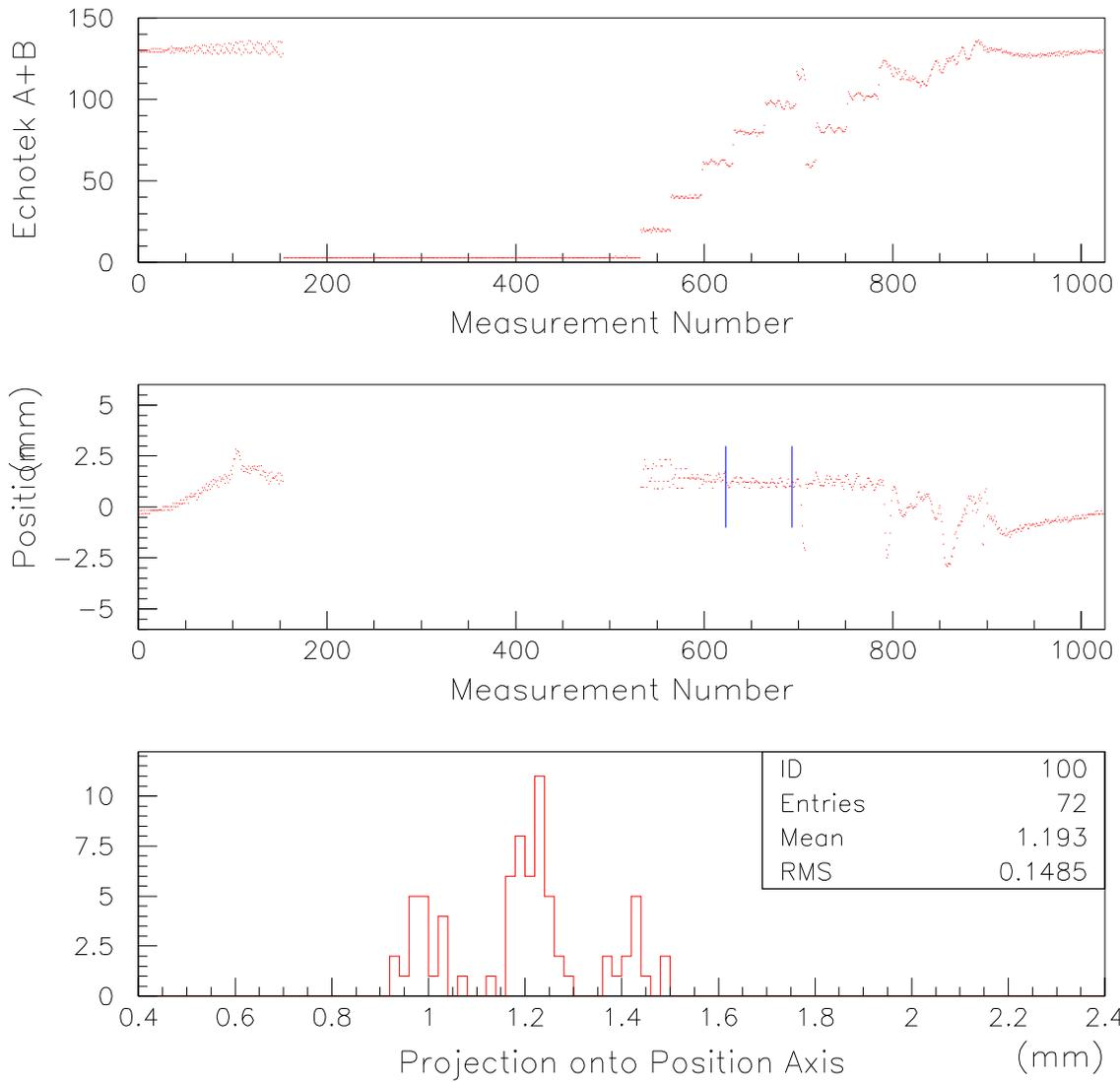
Figure 2: The upper two plots shows the same information as the previous plot but for a second data set. The vertical blue lines in the middle plot show the range of data selected to measure the position resolution. The bottom plot shows the projection of the data between the blue lines onto the position axis. The structure in this last plot will be investigated in the next figure.
