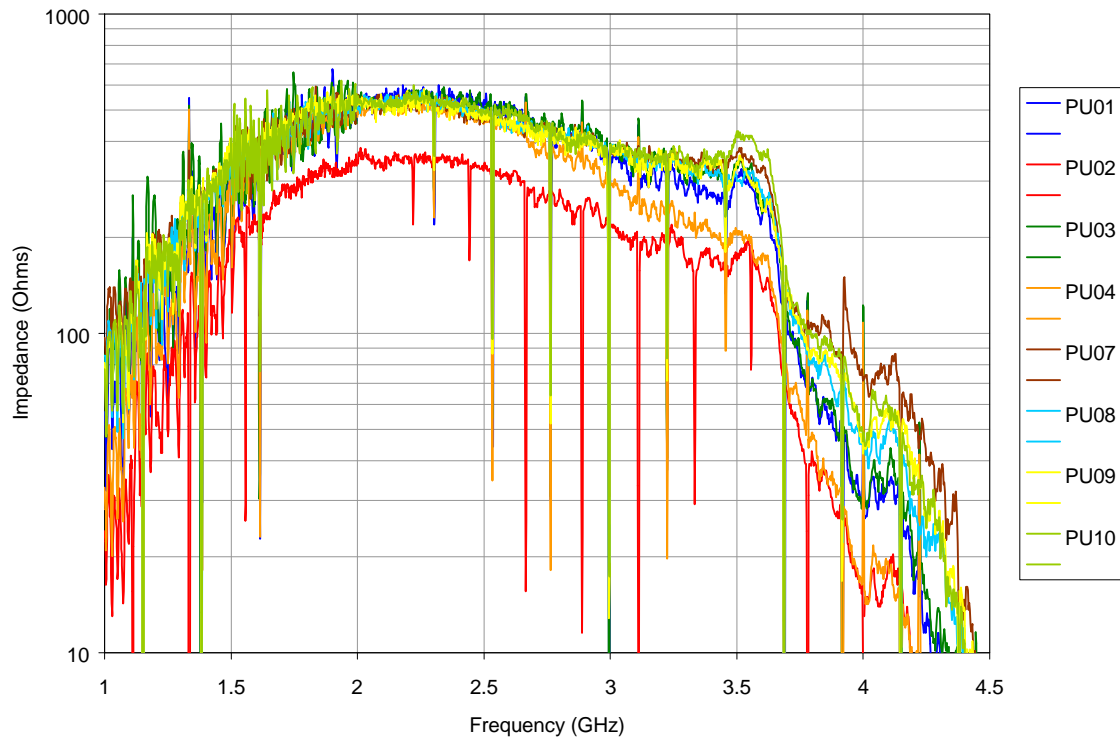
Figure 35. Pickup sensitivity of all arrays of Leg 1 of the 2-4 GHz StackTail System. There are 32 loops per array. A front-end noise temperature of 125 K was assumed.
