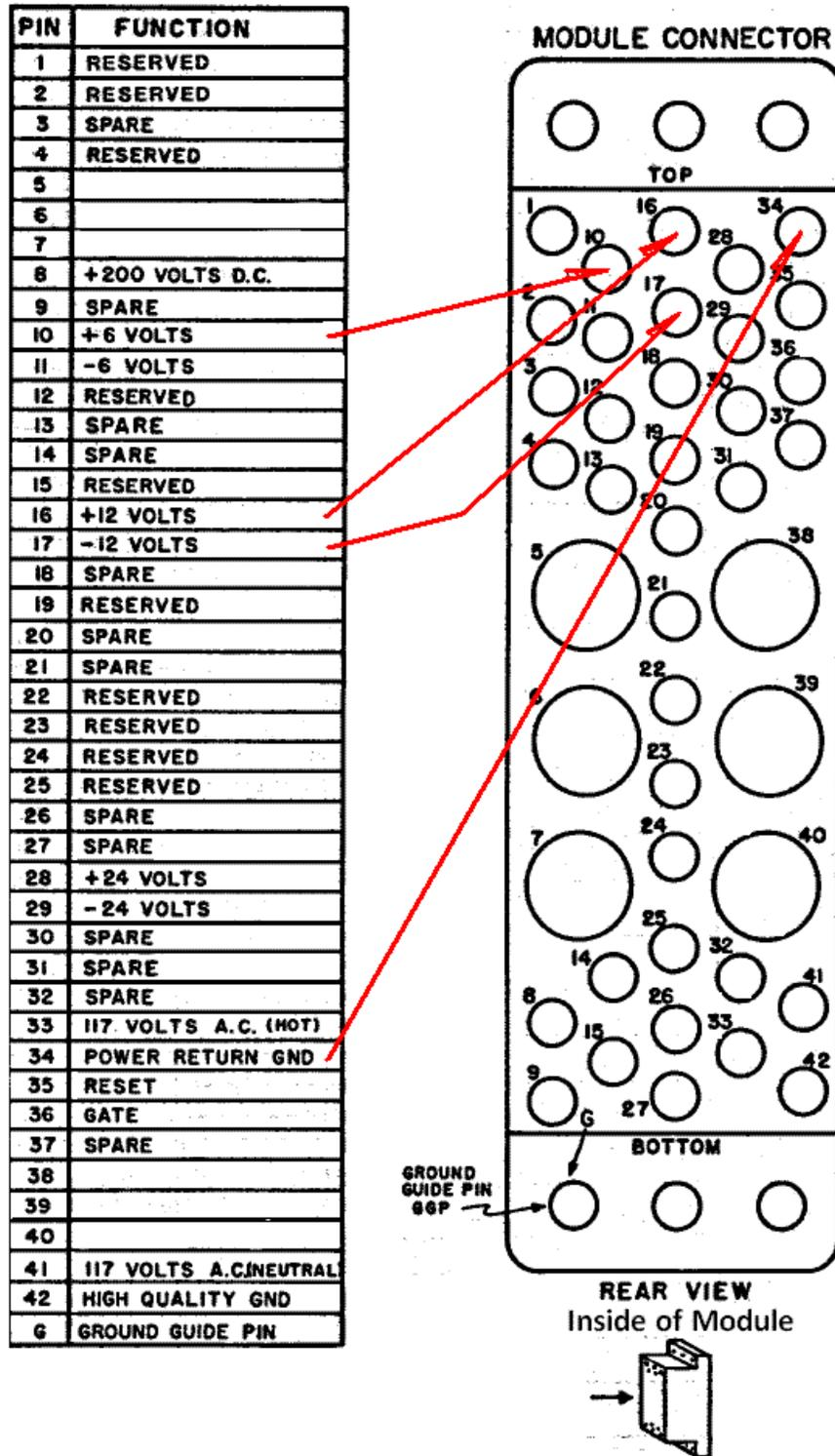
NIM power connector pin assignments.
