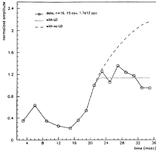
Fig. 2. Linear coupled-bunch theory vs. Booster data,  $n=16$ .
