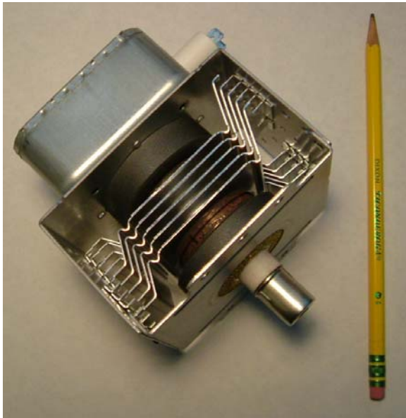
Photo of the CW, 1 kW magnetron type 2M219J
