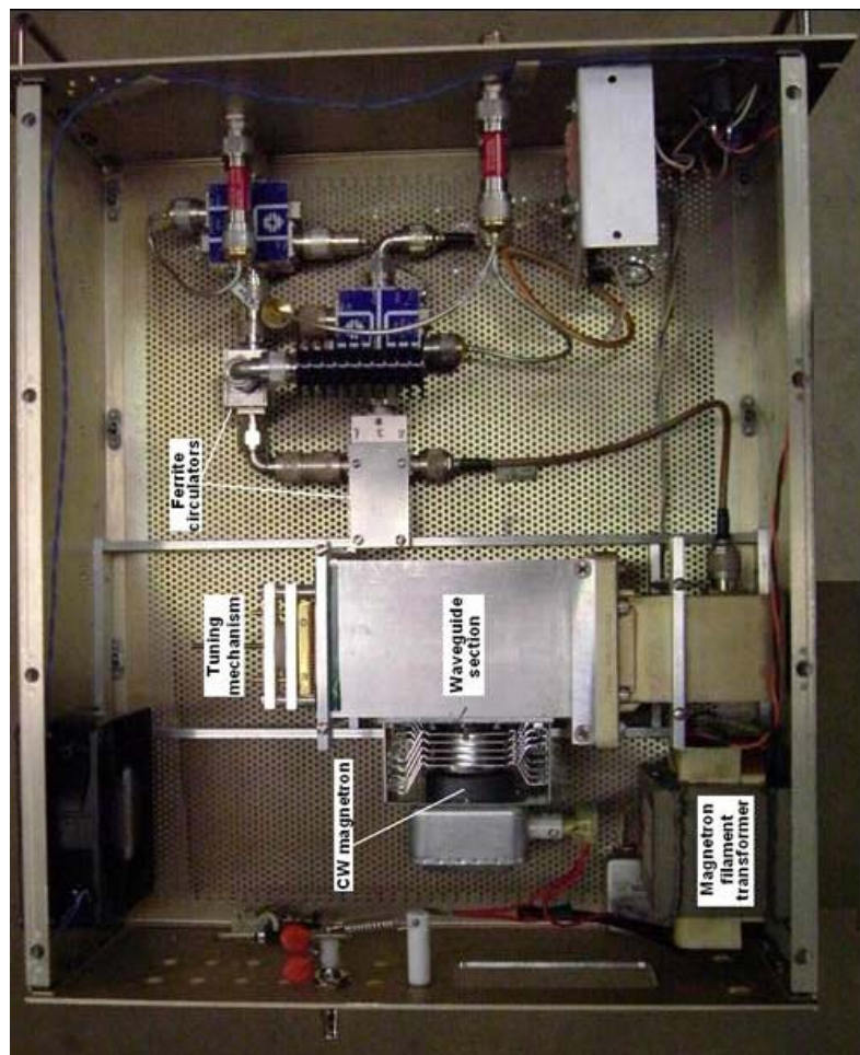
Module with a CW magnetron intended to work in injection-locked mode
