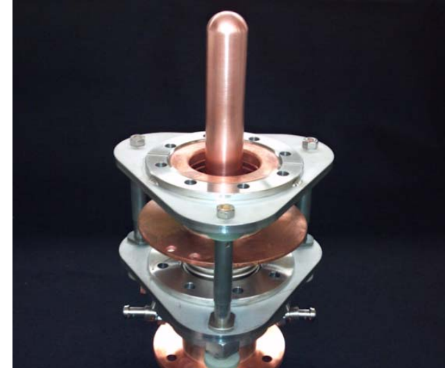
Rotating rod: Bakelite (Hall sensor attached) Rotation guide: Aluminum
