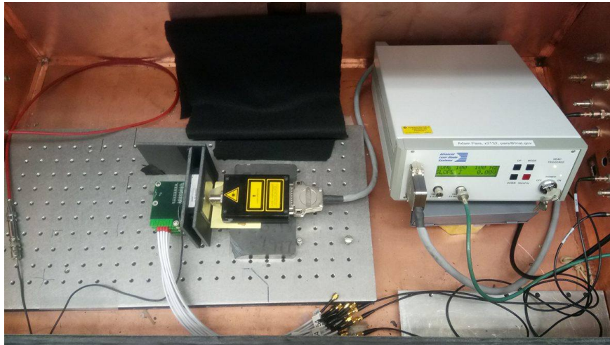
Figure 8: Experimental setup for laser tests, showing the MCP-PMT device (left), laser head (middle) and laser controller (right). Apparatus is situated inside a light-tight box.
