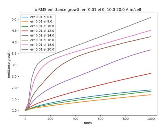
Emittance growth is larger for lens strength above 9 A-m.
