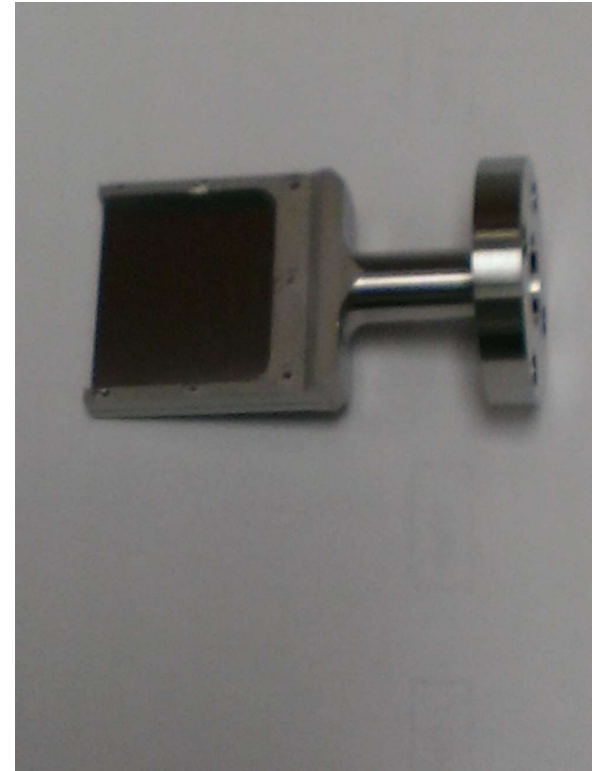
Primary Collimator (0.010" W) at 3 sigma on inside to scatter from x edge.
